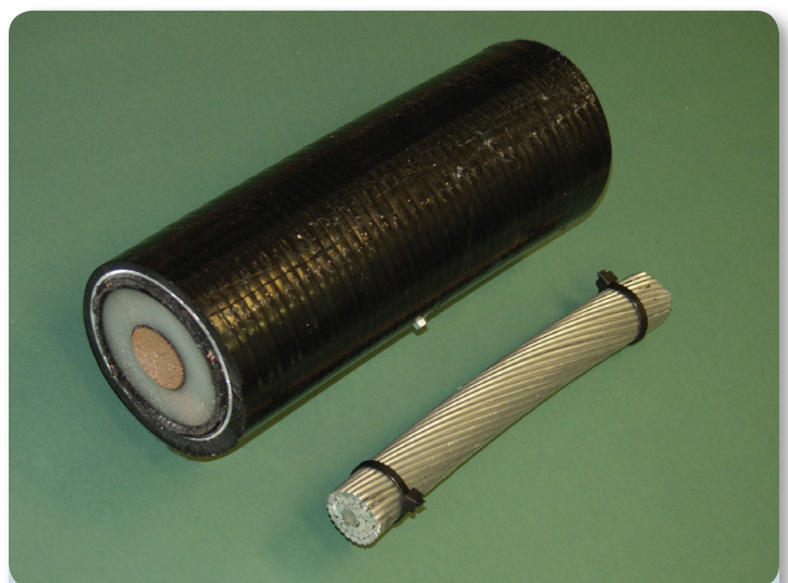
Underground cable and smaller overhead conductor.
