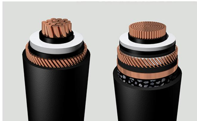
Figure on left is typical construction of a medium-voltage underground cable utilizing TR-XLPE solid insulation. Figure on right is typical construction of a high-voltage underground cable with PE-based semiconductive layers and super-clean XLPE solid insulation.
