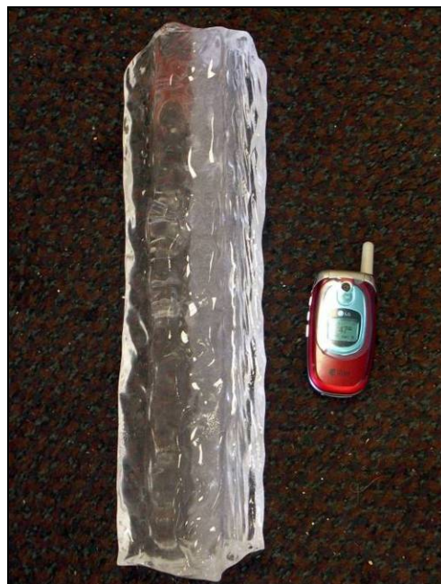
Figure 1.3: Illustration of Ice Accretion in Nebraska (Source: FEMA, 2008)
