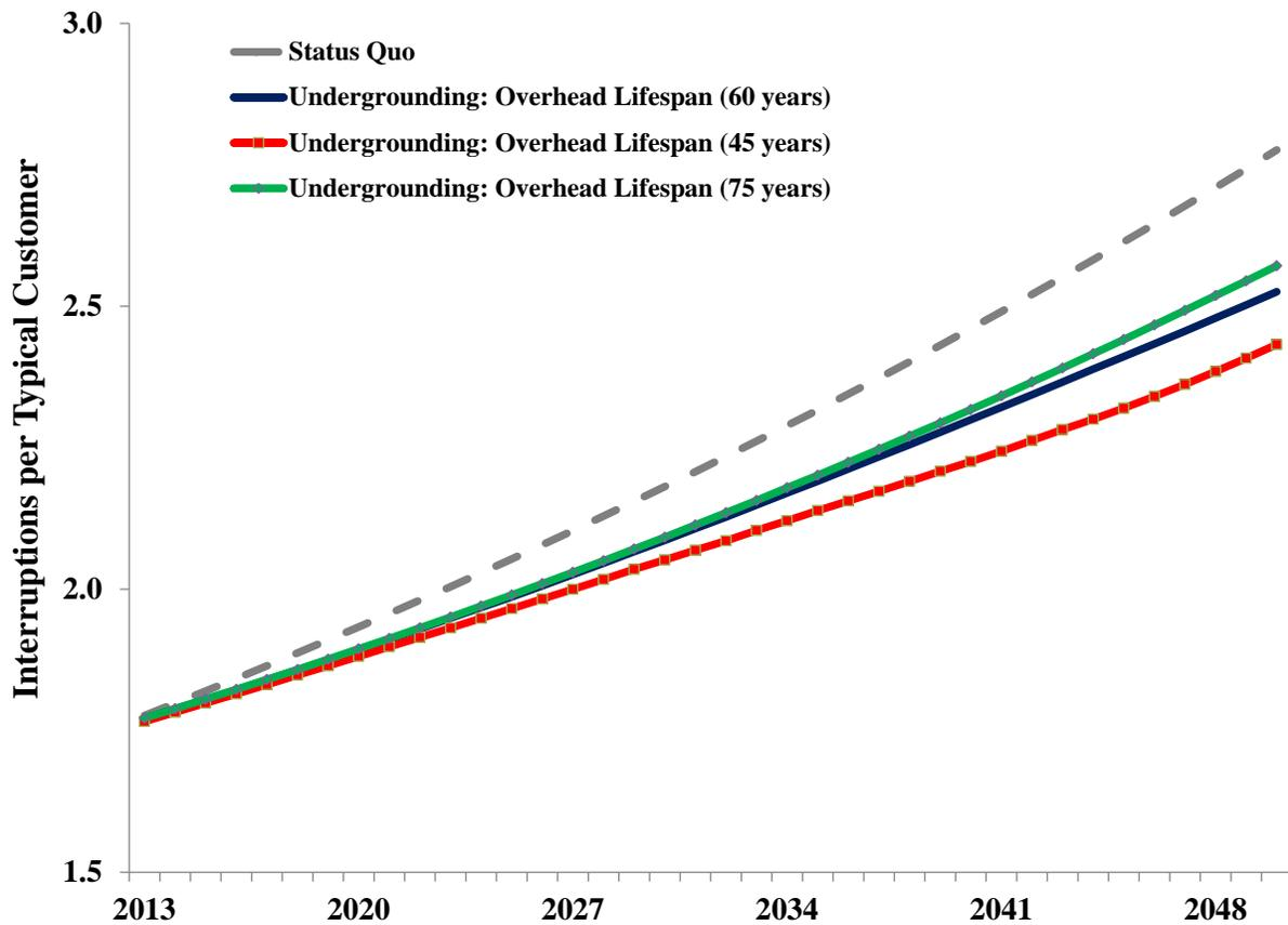
**Figure 6. Typical number of interruptions per customer for status quo and alternative assumptions about useful lifespan of overhead T&D lines**
