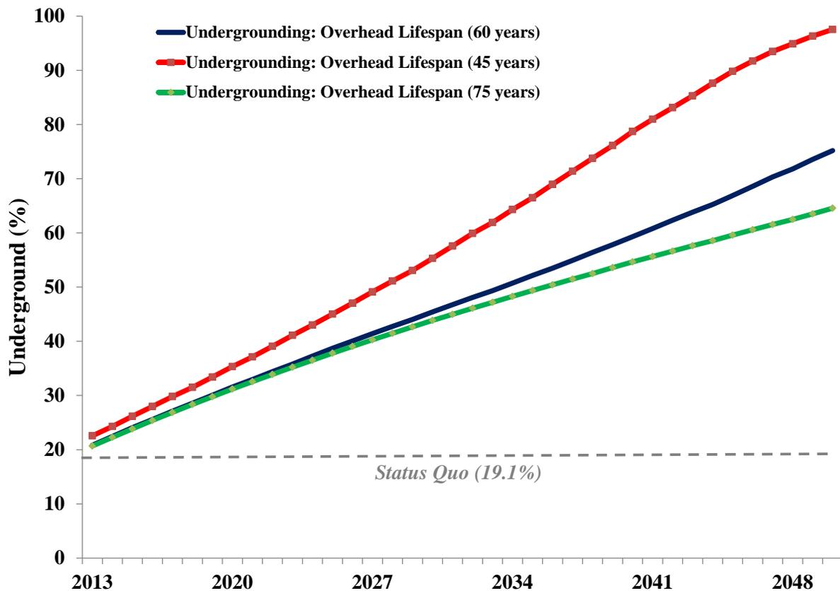
Figure 4. Share of underground line miles using alternative useful lifespans of overhead T&D lines
