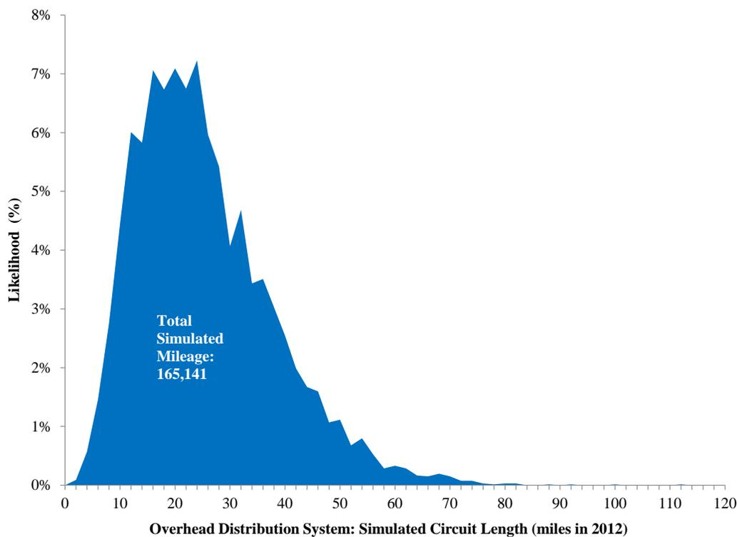
**Figure 3. Simulated mileage profile of Texas IOU overhead distribution lines**
