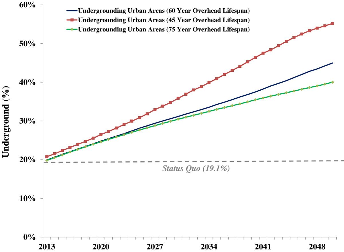
**Figure 12. Share of underground line miles using alternative useful lifespans of overhead T&D lines**
