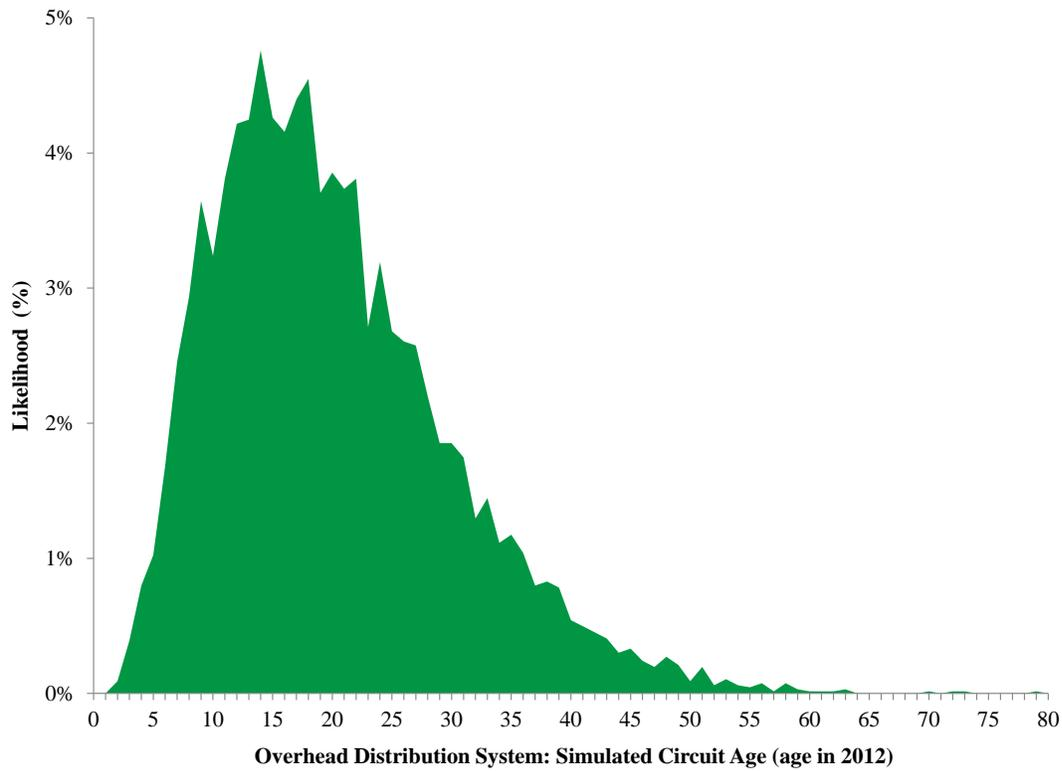
**Figure 2. Simulated age profile of Texas IOU overhead distribution lines**
